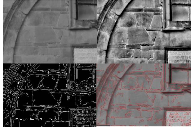
Figure 1. Original image (top left); image filtered with the Wallis filter (top right), edge extracted by the Canny operator (bottom left) and approximated edges used in the matching process (bottom right)
