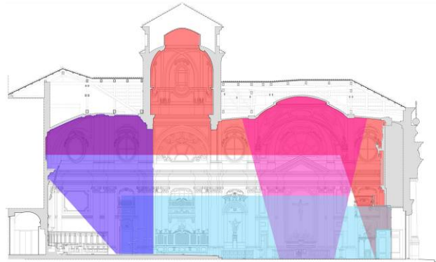
Figure 11: Surveyed surfaces in scan positions 1-2-3-4
