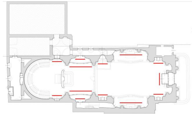
Figure 7: Positions of the images (red lines) subjected to the analytic photographic rectification process
